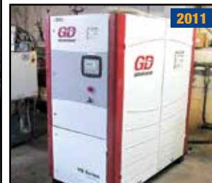
Gardner Denver VS-40A Air Compressor
